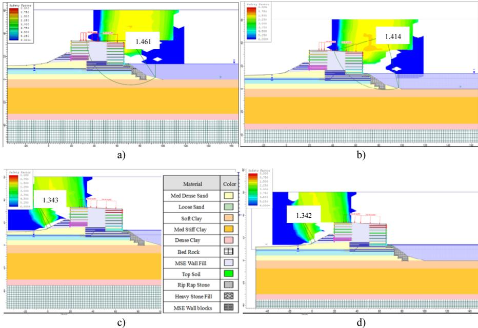
**Figure 5.** Results of the slope Stability at Station 28 at high water condition a) Right Abutment Bishop's Method b) Right Abutment Spencer Method c) Left Abutment Bishop's Method d) Left Abutment Spencer Method.
