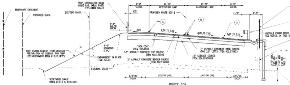
Figure 2. Initial section close to the bridge.
