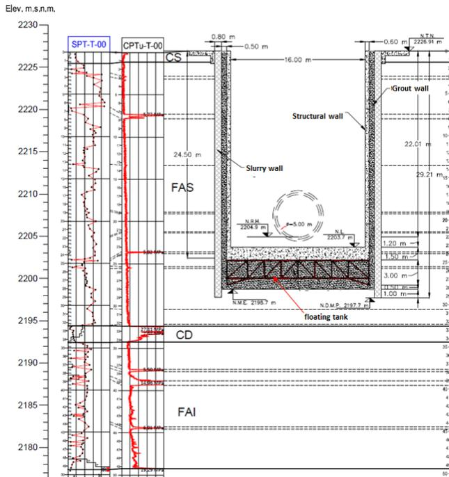
Figure 2. Stratigraphy of the site under study and geometry and tunnel shaft elements in study case.
