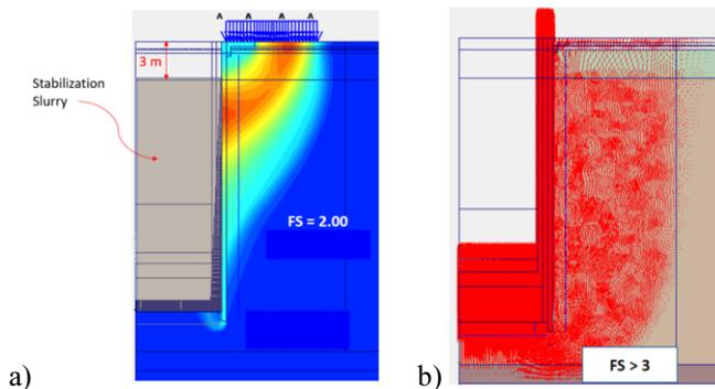
**Figure 6.** a) General failure mechanism and b) Failure mechanism with buoyancy condition.
