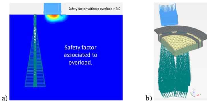
**Figure 7.** a) Panel analysis with 3D FEM and b) failure mechanism in the panel excavation.
