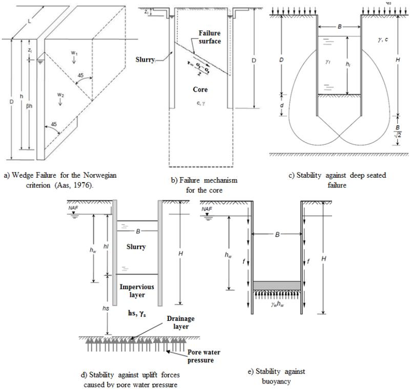
Figure 4. Failure mechanisms and analysis schemes (Modified from [1]).
