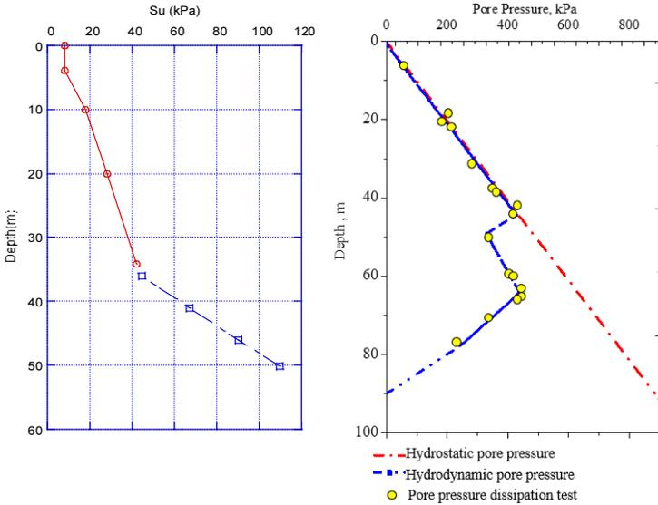
Figure 1. a) Pore water pressures at the study site and b) Undrained shear resistance envelopes ( $S_u$ ).
