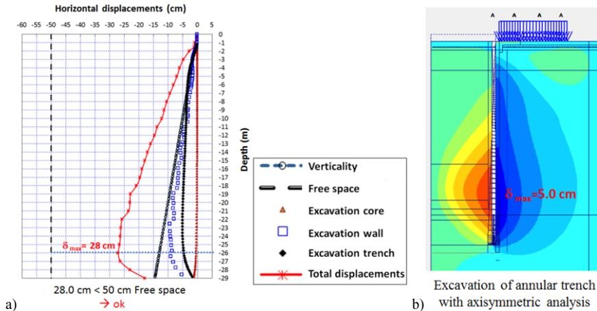
**Figure 8.** a) Cumulative displacements for the wall with the verticality deviation and b) displacements contour for excavation trench.
