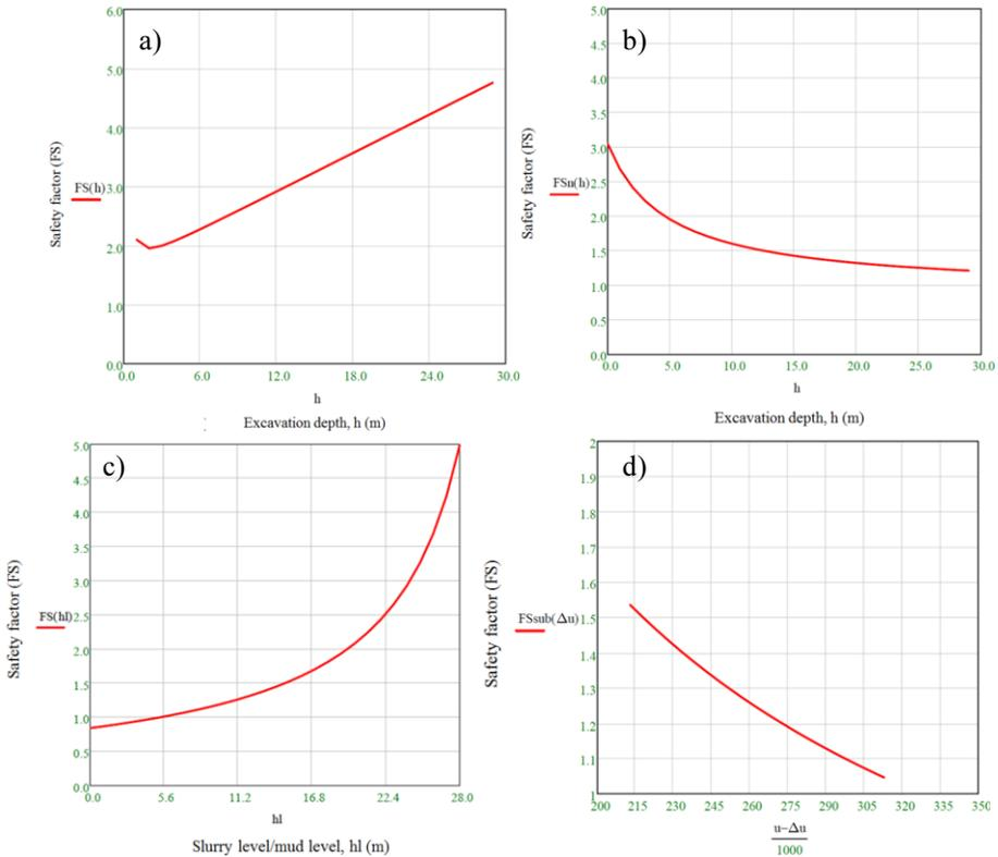
**Figure 5.** a) Plot of safety factor against the excavation depth of the slip wedge; b) safety factor of the core stability against the depth of the trench; c) Plot of safety factor against slurry height and d) Plot of safety factor against relieved pore water pressure.
