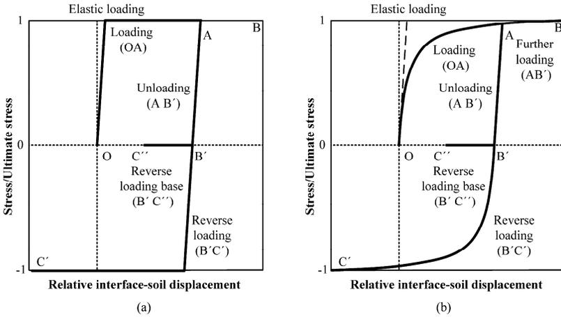
Figure 2. (a) Elastic perfectly-plastic and (b) nonlinear elastoplastic behaviour of the interface and the near-pile soil.
