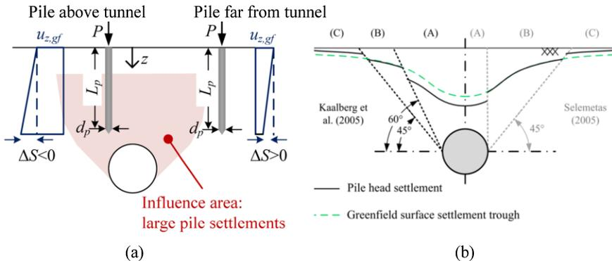
**Figure 1.** (a) Sketch of the tunnel-pile interaction problem and greenfield ground movements,  $u_{z, gf}$ . (b) Relationships between pile and greenfield surface settlements depending on the pile tip location [12].
