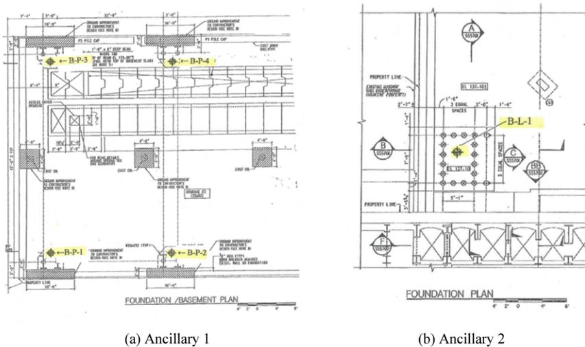
**Figure 1.** Foundation layout and geotechnical borings at Ancillary 1 and 2.
