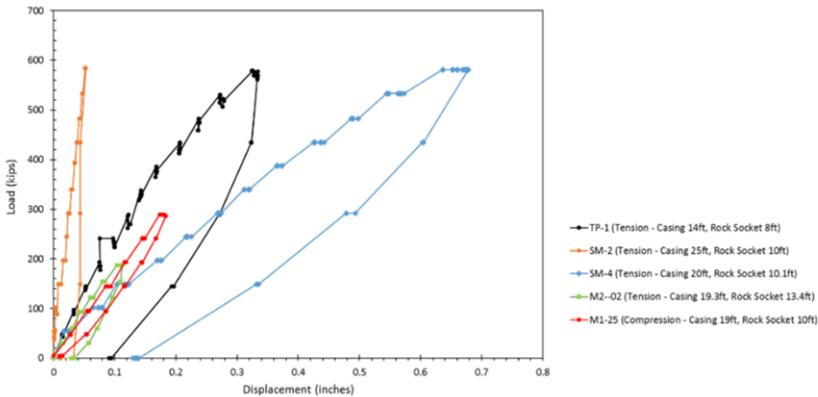
Figure 4. Applied load versus displacement at top of test pile.
