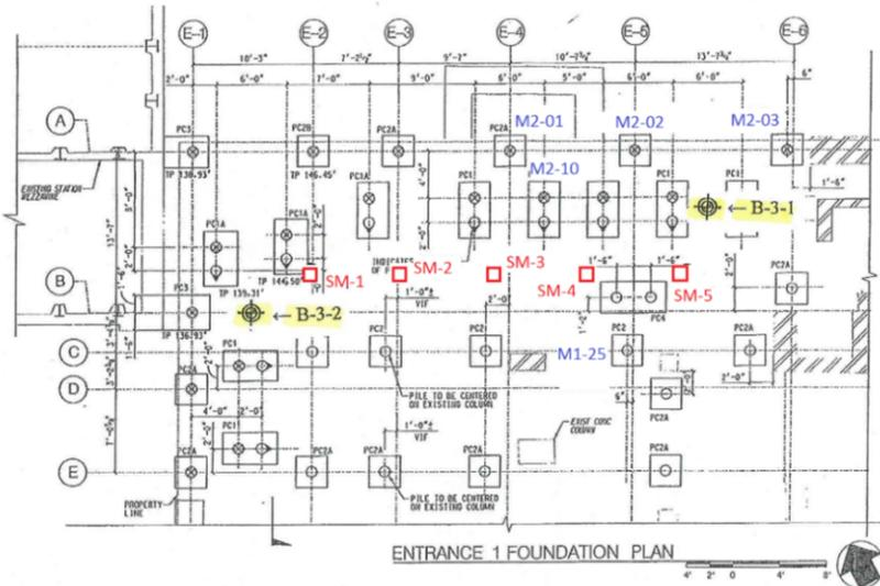
Figure 2. Foundation layout and geotechnical borings at Entrance 1.
