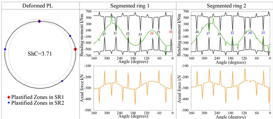
Figure 5. Results on the primary lining.
