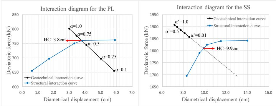
Figure 4. Interaction diagrams for the analysis without causeway.
