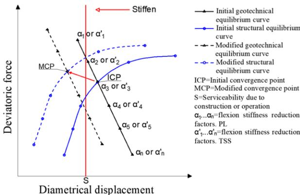
**Figure 1.** Geotechnical-structural convergence for segmented and double lining tunnels.
