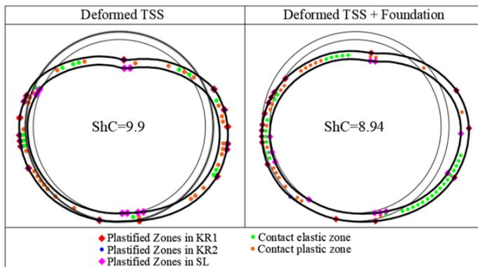
Figure 7. Distorted and plastic points for the SS without causeway and with causeway.
