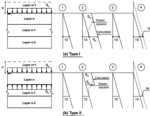
**Figure 5.** Modelling of the vertical stress load–unload cycles verified during the compaction of the backfill layer, using compaction procedures types I and II.
