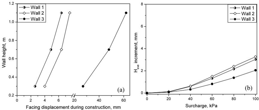
Figure 3. Horizontal facing displacement (a) during construction and (b) post construction.
