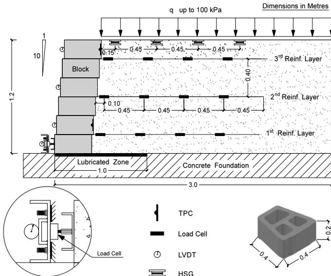
Figure 1. A cross-sectional view of a block face wall.
