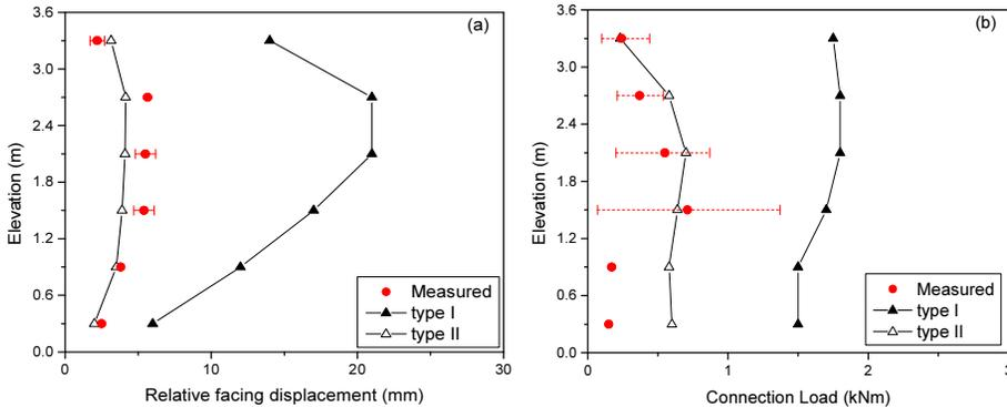
**Figure 6.** Measured and calculated values of the a) horizontally-facing displacement at the end of construction and b) connection load.
