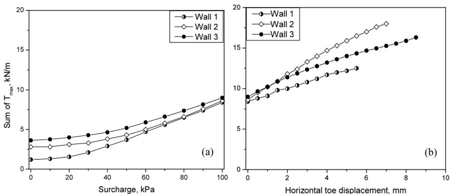
Figure 2. Sum of maximum reinforcement load (a) during surcharge application and (b) toe release.
