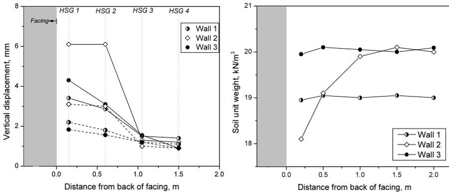
**Figure 4.** Vertical displacement at the end of surcharge application, EOL (dashed lines), and toe release, EOR (solid lines) and backfill soil unit weight for three walls.
