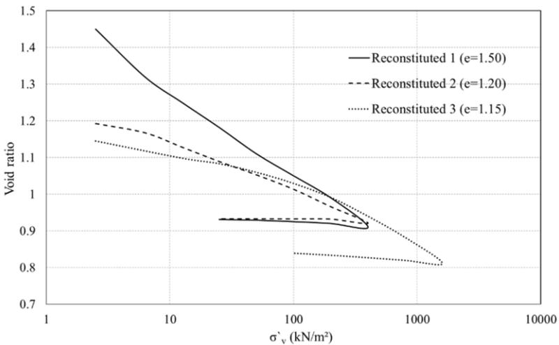
Figure 2. Consolidation curves for gold tailing specimens.
