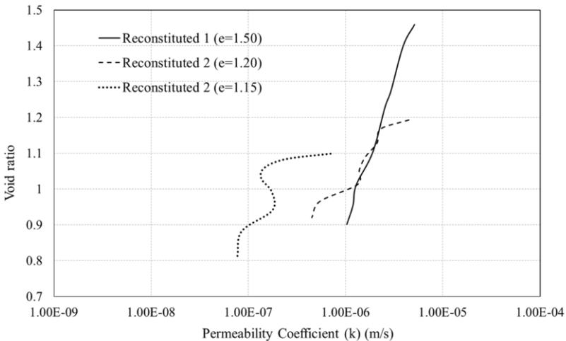
Figure 4. Permeability coefficient versus void ratio for gold tailing specimens.
