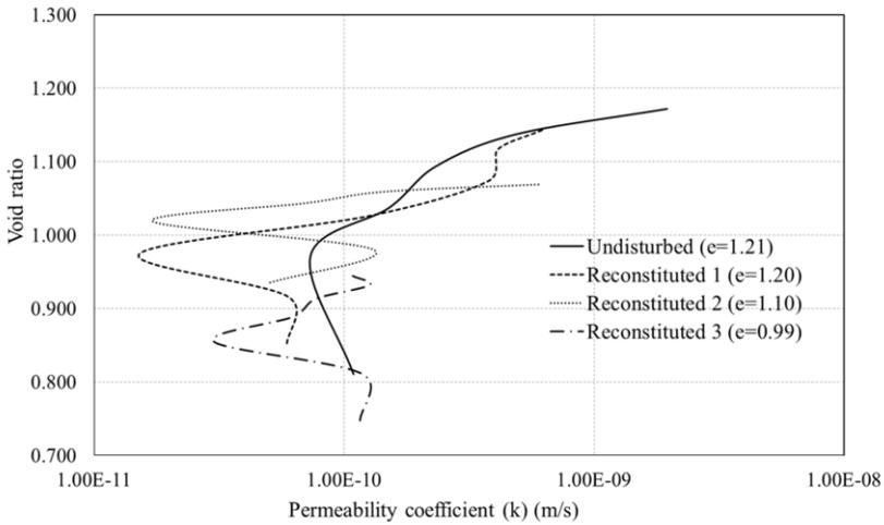
Figure 3. Permeability coefficient versus void ratio for bauxite tailing specimens.
