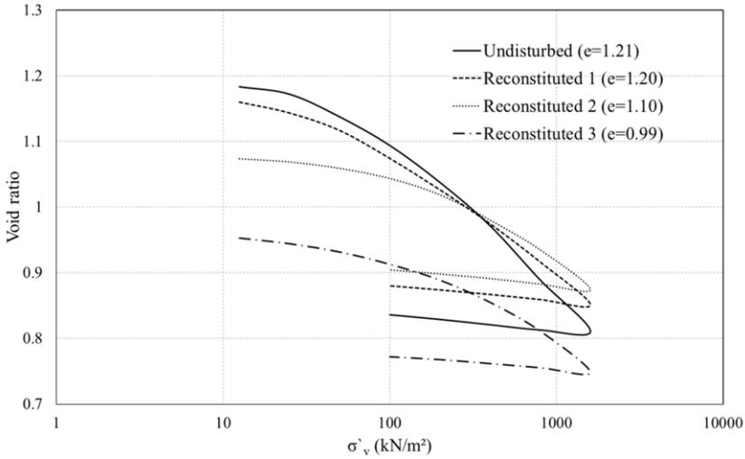
Figure 1. Consolidation curves for bauxite tailing specimens.
