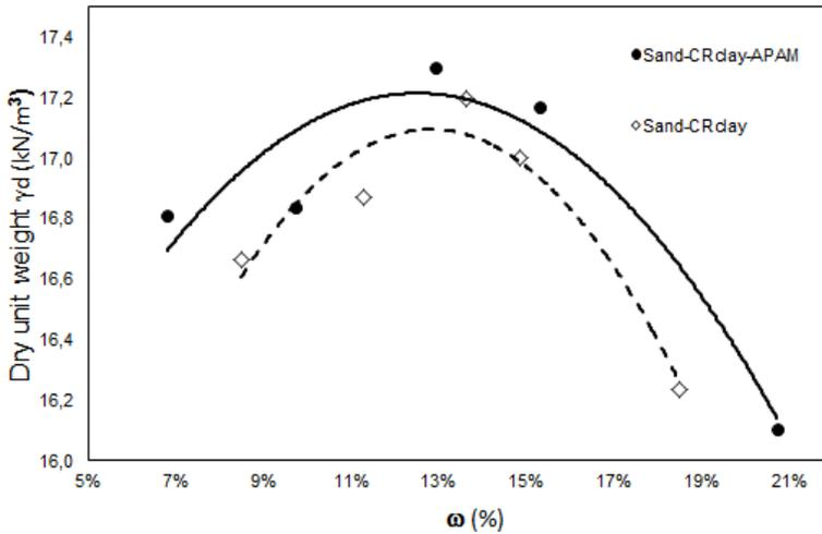
Figure 2. Standard Proctor test on sand-CRclay and sand-CRclay-APAM.
