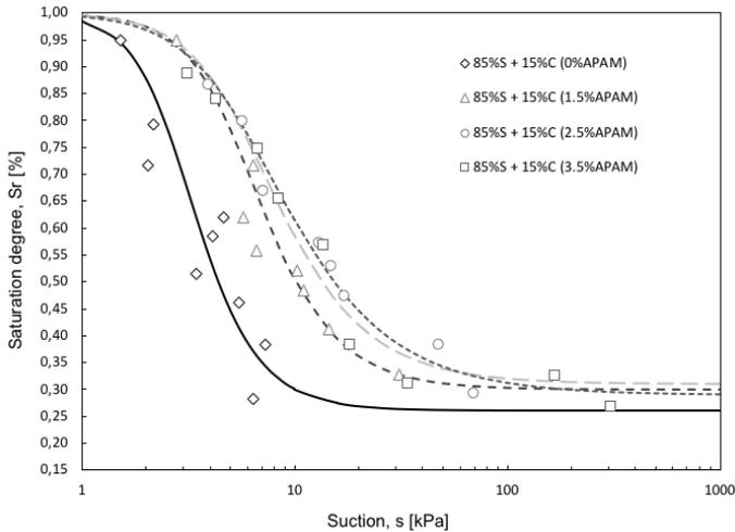
**Figure 5.** Experimental values of suction and saturation degree for different polymer content in sand – CRclay mixtures (dot) and calibration of van Genutchen equation (lines).
