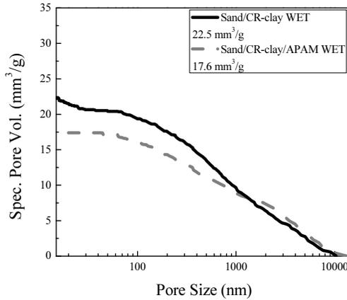
Figure 4. Pore size distribution of sand-CRclay & sand-CRclay-APAM with different moisture.
