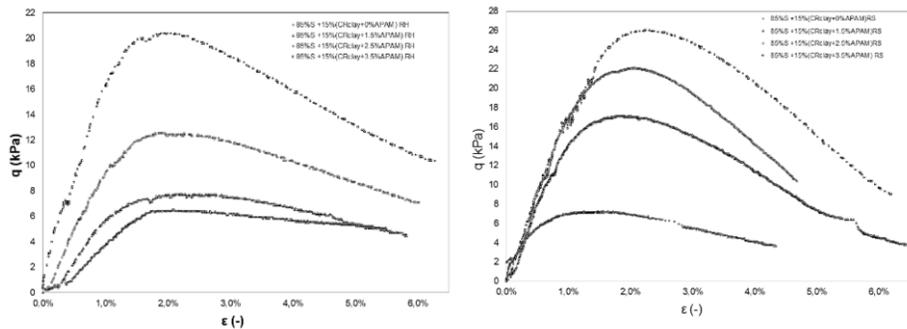
**Figure 3.** UCS curves for dry (RS) and wet (RH) side on sand-CRclay-polymer mixture. Mixtures vary the percentage of APAM from 0% to 3,5%.
