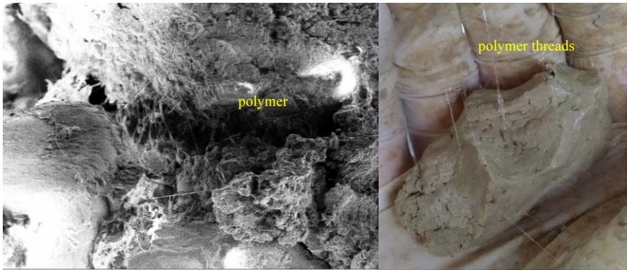
**Figure 1.** a) Microscopic inspection on soil- polymer mixture by SEM. b) Macroscopic inspection on Clay-polymer mixture after changing its moisture content.
