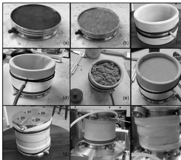
Figure 2. Specimen preparation and test procedure.
