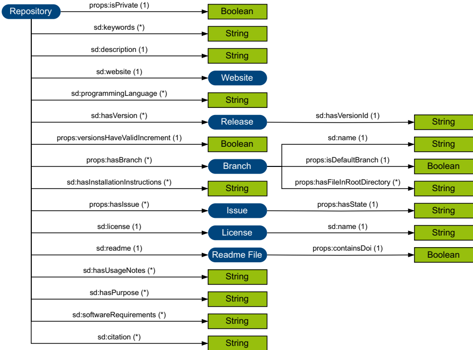
Figure 3. An abstract visualization of the ontology underlying the repository representations (data graphs). IRIs are depicted in blue, literals in green. The cardinality is given in brackets. sd refers to the Software Description Ontology namespace, and props to the namespace for additional custom properties.
