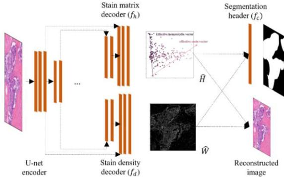
**Figure 1.** Multi-decoder Unet architecture for joint multi-task learning
