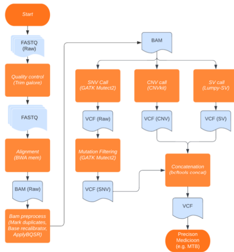
Figure 2. Workflow of Onkopipe. Onkopipe analysis steps generally follow the National Cancer Institute Genomic Data Commons (GDC) bioinformatics pipeline and the best practice guidelines published by the Broad Institute. It includes the use of Trim Galore for quality control, BWA mem for alignment, Picard MarkDuplicates to remove duplicates, and GATK for base quality score recalibration. The SNV, CNV and SV variants were called using GATK mutect2, CNVkit, and LUMPY-SV, respectively and concatenated into a unified VCF as output. Additional SNP calling (HaplotypeCaller, GenotypeGVCFs) and annotation (VariantAnnotation) steps are only used for evaluation, thus they are not shown in the flowchart.
