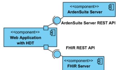
Figure 1. System's component diagram.
