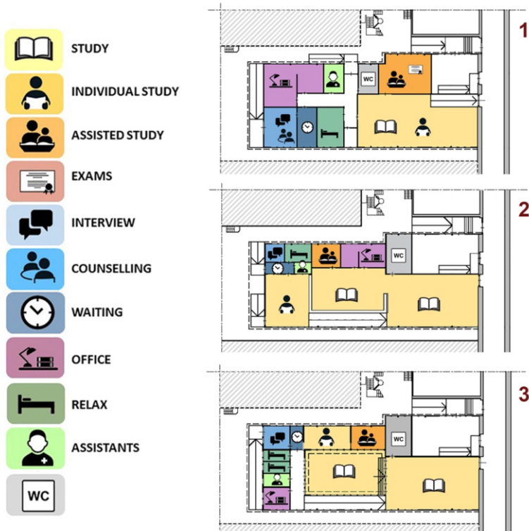
Figure 4. comparison between the 3 distribution layouts developed in the refurbishment of the existing building to be adapted to a new pole for the Special Needs unit
