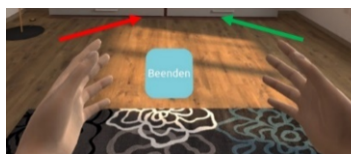
Figure 3. Hand movement direction with mirror mode activated. If the controller is in right hand and move towards left (green arrow), the left hand will move towards right (red arrow).
