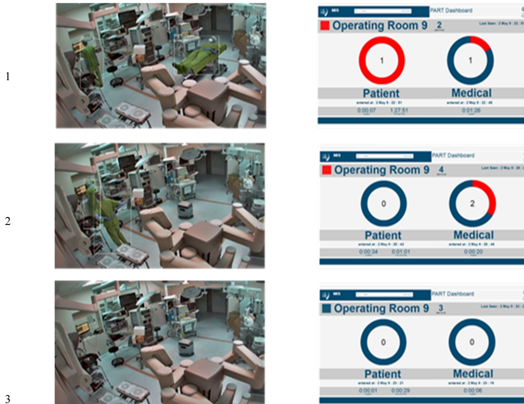
Figure 2 – OR State computation based on AI driven video stream analytics and complex event processing. Each row includes two images. On the left the video stream and the detected object class of the AI is shown by a white rectangle. On the right the dashboard shows the resulting state of the OR and the computed utilization figures. State 1: The patient (circle lights up red) and one medical professional (circle lights up red proportionally) are detected. State 2: Two medical professionals are currently in the OR. State 3: The room is empty and shown as inactive (blue square in the upper left corner). Note, as soon as the patient or the last medical professional left the length of stay is computed and depicted in the dashboard.
