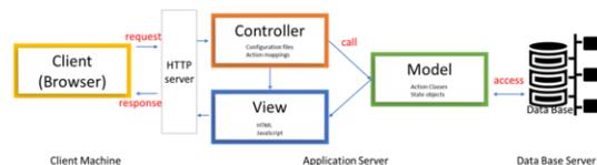
Figure 1– Three tier MVC architecture
