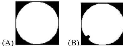
**Figure 7.** (A) Clear hole. (B) defective hole.
