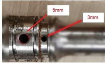
**Figure 1.** The two sizes of shaft holes.
