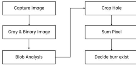
**Figure 4.** Image processing flow for the burr inspection system.
