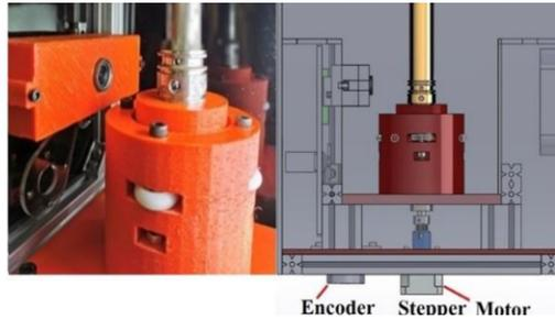
**Figure 2.** The fixture for supporting and locating the shaft.
