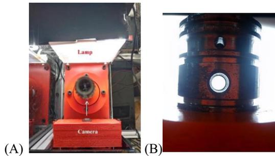
**Figure 3.** (A) Image acquisition device, (B) Image from the device.
