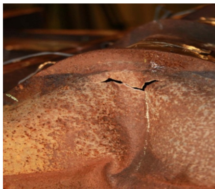
Figure 6: Plastic hinges and plate tearing, severely corroded box girder [32].
