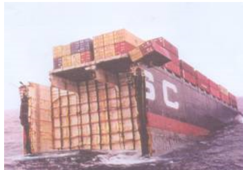
Figure 4. Complete brittle hull girder failure of the container vessel MSC Carla
