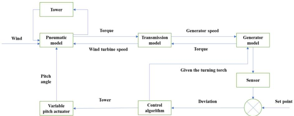
Figure 1. Structure of wind turbine control system
