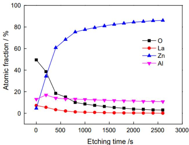
Figure 2. XPS depth analysis chart with processing time of 1 min
