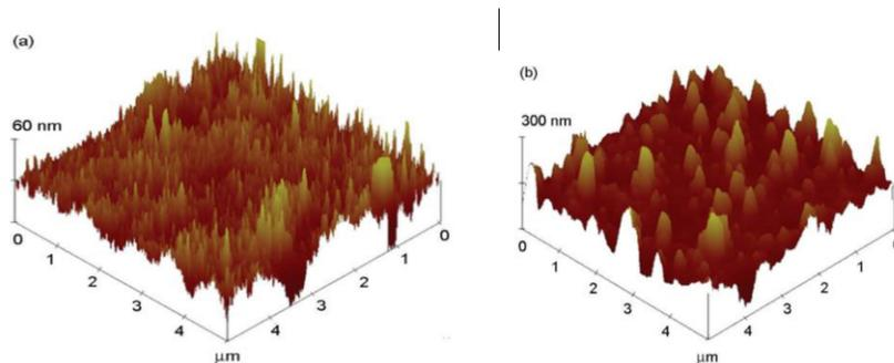
Figure 3. AFM diagram of lanthanum salt conversion film sample of Galfan coating.
