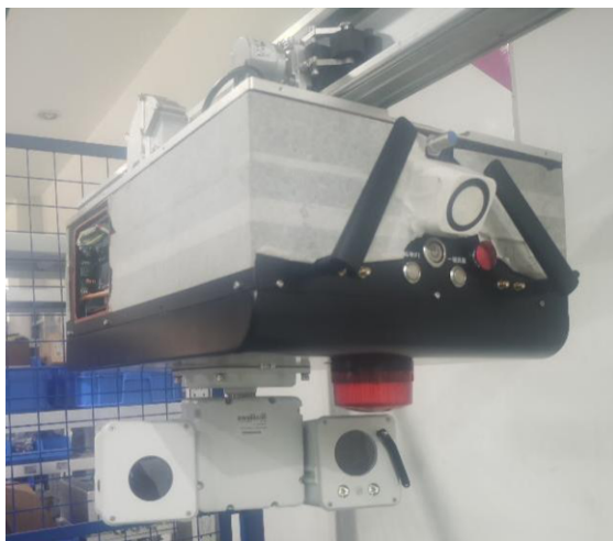
Figure 7. Safety intelligent inspection system for coal terminal conveying equipment
