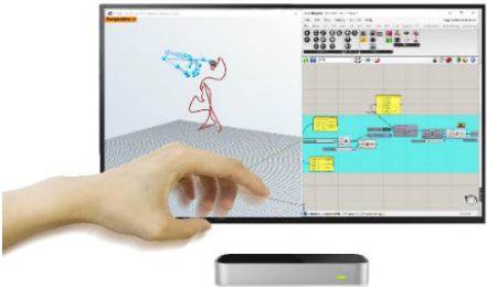
Figure 5. Leap Motion reads gesture trajectories. (Left)
