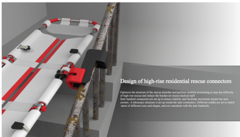
Figure 5. Design of high-rise residential rescue connectors.
