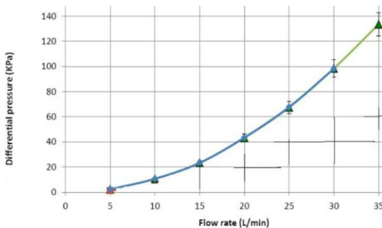
Fig. 6 Warm air flow resistance curve
