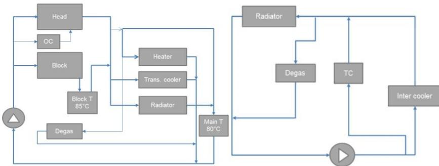
**Fig. 2** Schematic diagram of cooling system principle
