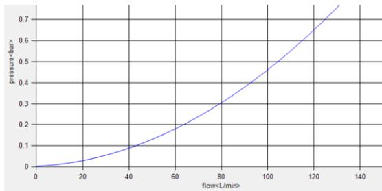
Fig. 5 Flow resistance curve of radiator
