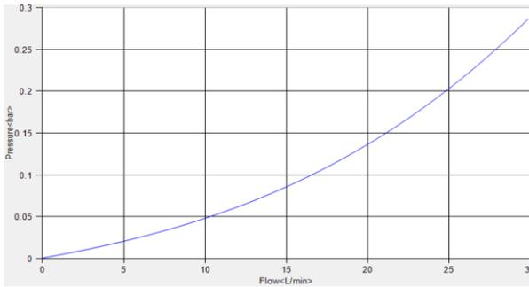
Fig. 8 Flow resistance curve of the oil cooler
