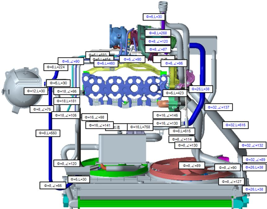
Fig. 10 Cooling system connection pipeline
