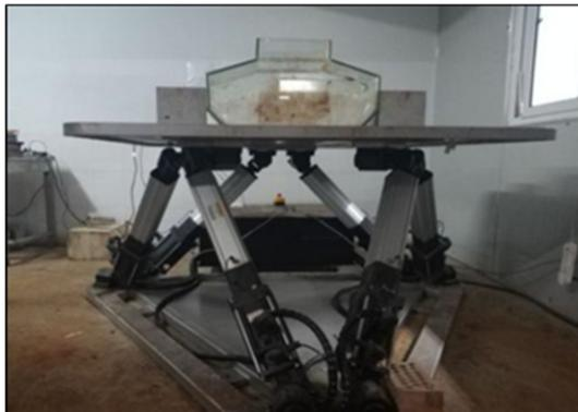
**Figure. 1** Six degrees of freedom shaking table and cargo hold model.
