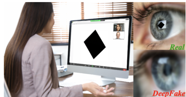
Figure 8. Video conferencing DeepFakes detection [39]. Left: A video call attendant is being actively authenticated with the live patterns shown on the screen. Right: A real person's cornea will produce an image of the pattern shown on the screen while a real-time DeepFake cannot.
