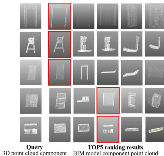
**Figure 6.** TOP5 ranking results. The queries are 3D point cloud components, and the ground truths and correct retrieval results of BIM model point cloud components are labeled with the red bounding boxes.
