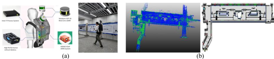
**Figure 2.** The backpack mobile LiDAR scanning equipment.
