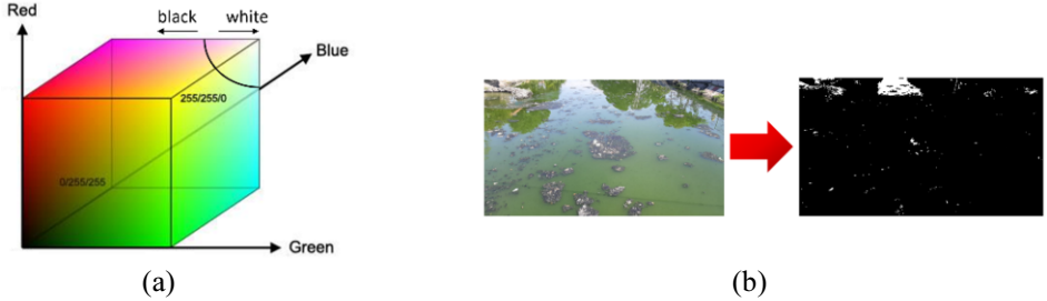
Figure 24. Color filtering: (a) closer the white inside the RGB color space, and (b) result of color filtering
