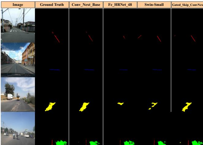
**Figure 2.** Segmentation results of different models. Each row presents a different crack—row1: Longitudinal Crack, row2: Transverse Crack, row3: Alligator Crack, and row4: Pothole.
