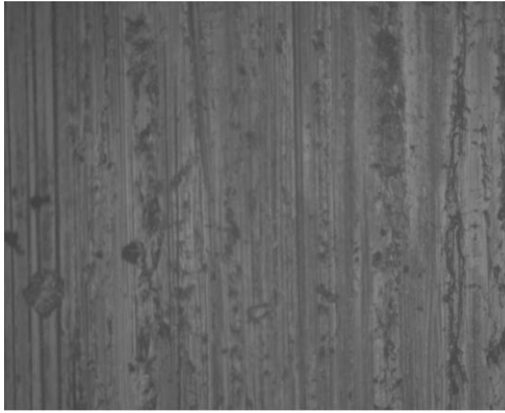
Figure 4. Surface morphology under the load of 130 N, rotational speed 230 r/min, and hardness 282 HV.
