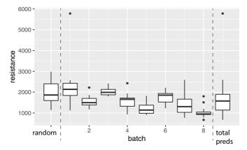
**Figure 6.** Quality of produced graphene (resistance in  $\Omega$ ) for patterning lines from graphene oxide on quartz (GOQ), lower is better. On the left of graph, the distribution of resistance for the initial training data is shown. We show results summarized by batch of 14 lines; each boxplot represents one batch. The boxplot on the right of the graph shows the distribution of measured resistances for all configurations that the MBO explored.
