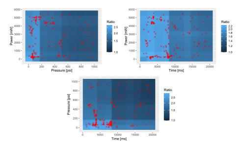
**Figure 5.** Partial dependence plots for pairs of continuous parameters of the predictions of a surrogate model trained on all available data for GOQ. Red crosses denote parameter configurations that were evaluated experimentally and are concentrated in the areas with the best predicted G/D ratios.
