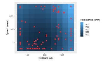
**Figure 7.** Partial dependence plot for patterning speed and pressure in the reaction chamber of the predictions of a surrogate model trained on all available data for patterning lines. Red crosses denote parameter configurations that were evaluated experimentally.
