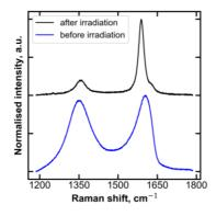
**Figure 2.** Raman spectra showing D (left peak) and G (right peak) bands of graphene oxide before (bottom) and after (top) laser irradiation. The ratio we optimize in this paper is calculated from the area under the peaks. The intensity is shown in arbitrary units (a.u.).
