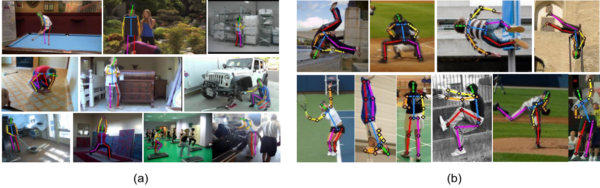
Figure 6. (a) Examples of estimated poses on the MPII Human Pose test dataset. (b) Examples of estimated poses on the LSP test dataset. Our model deals well with occlusions, blurred and twisted limbs, abnormal poses, and changes of view position.
