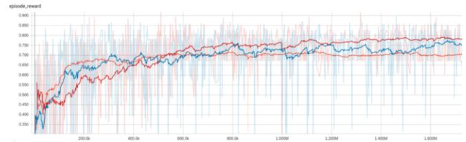
**Figure 6:** Training progress of the LDGCNN (blue), the voxel based network (orange) and the PointNet (red). The vertical axis represents the achieved reward. The horizontal axis represents the time steps.
