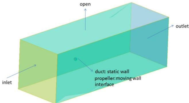
**Figure 6.** Boundary conditions for numerical analysis of ducted fan
