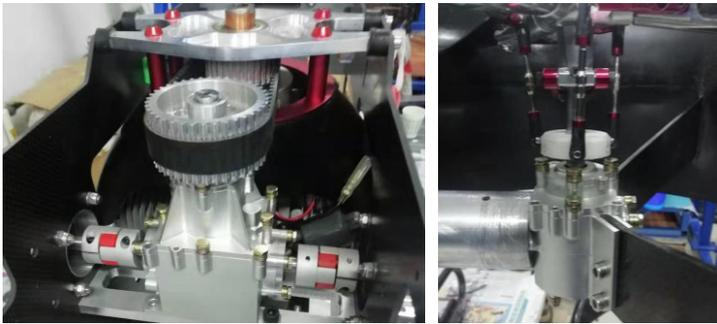
**Figure 10.** Mounting of transmission system gearboxes
