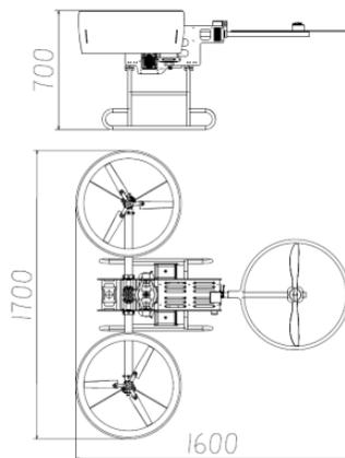
**Figure 2.** Dimensions of ducted fan UAV
