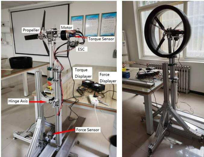
Figure 7. Ground test platform for ducted fan
