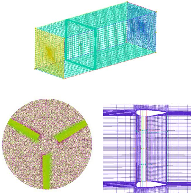
**Figure 5.** Mesh for numerical analysis of ducted fan
