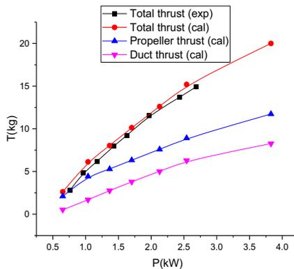
Figure 8. Power vs. thrust of the ducted fan.
