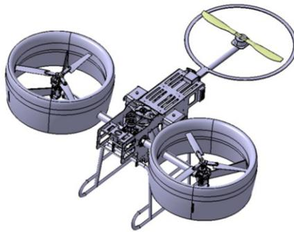
**Figure 1.** Configuration of ducted fan UAV
