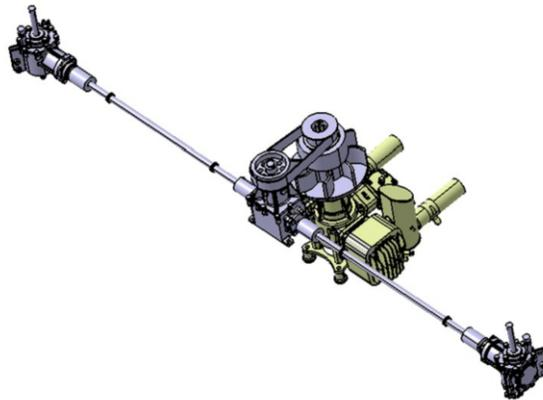
**Figure 3.** Transmission system of ducted fan UAV
