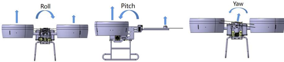
**Figure 4.** Control concept of ducted fan UAV
