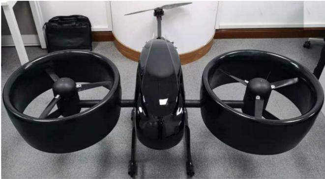
**Figure 9.** Full-scale prototype of ducted fan UAV
