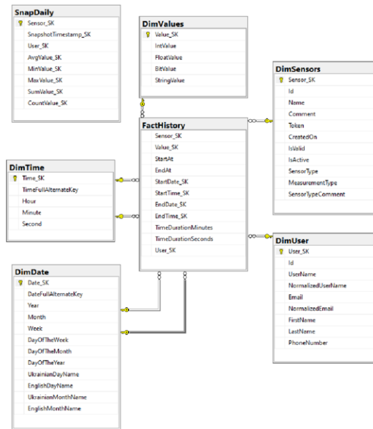
Figure 2. Optimized star schema design for IoT analytical data warehouse (Azure Synapse), with fact and dimension tables for historical analysis, and SnapDaily for daily aggregated smart home metrics
