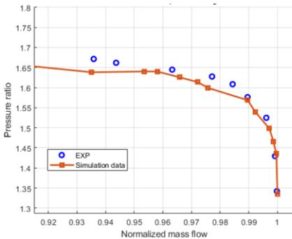
**Figure 3.** Rotor67 Total pressure ratio curve
