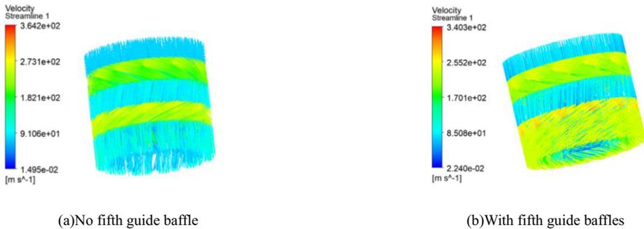
Figure 11. Lift fan 3D velocity field flow diagram
