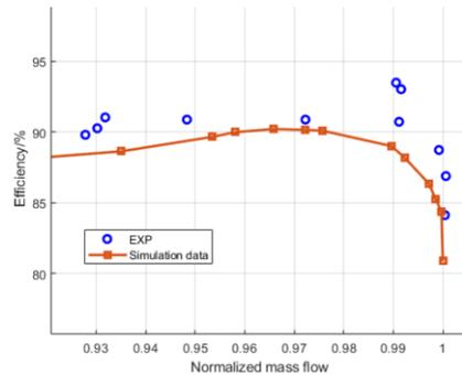
**Figure 4.** Rotor67 Efficiency curve
