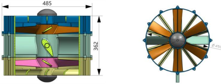
Figure 1. Schematic diagram of lift fan structure
