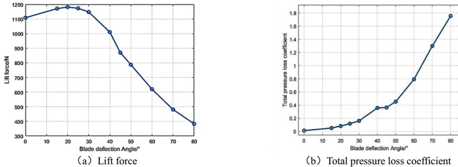
Figure 8. Effect of Inlet Guide Vane Deflection on Lift and Pressure Loss in Lift Fans.
