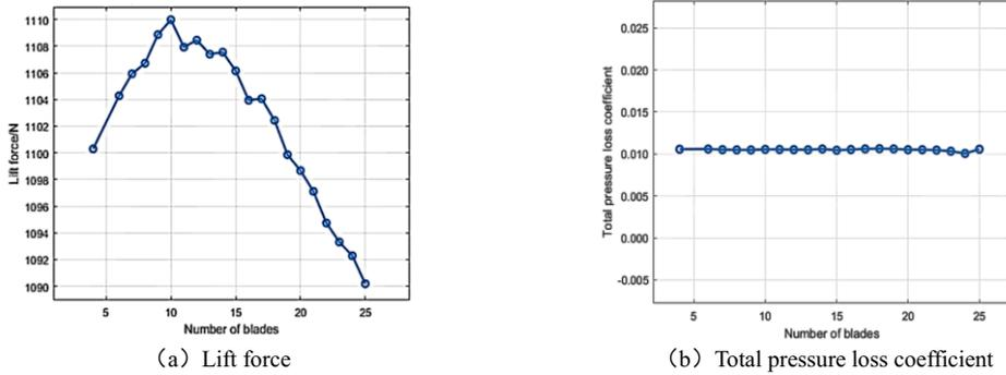
Figure 7. Inlet Guide Vane Count Effects on Lift and Pressure Loss in Lift Fans
