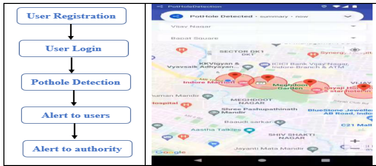
Figure 5. (a) Flow chart of User Interface, (b) Potholes marked on the given route map and notification comes before the pothole arrives
