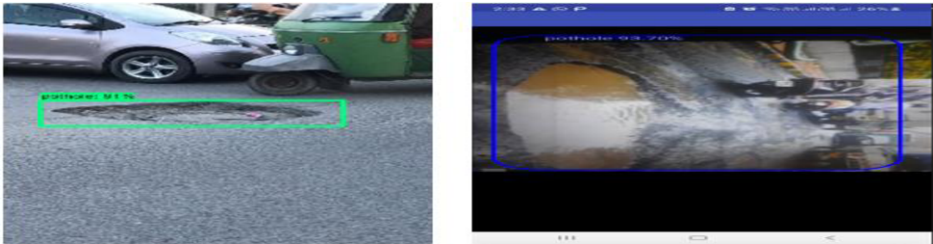
Figure 3. Pothole detection through SSD on a route with (a) 91% confidence interval and (b) 93.70% confidence interval
