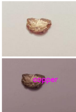
Figure 4. Messing detected as copper
