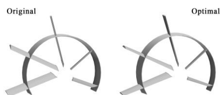
Figure 6. The pre-swirl fairing before and after optimization.
