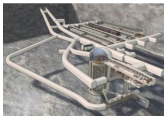
Figure 1. 3D diagram of the Swedish SFR repository (Phase I).
