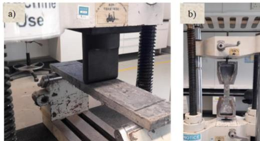
Figure 2. (a) Flexural strength test (b) Tensile strength test.
