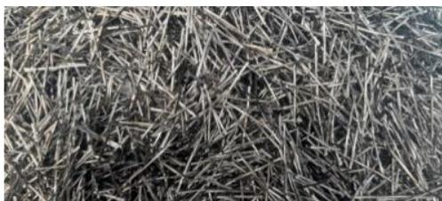
**Figure 1.** Macro Basalt Fibre (MBF).
