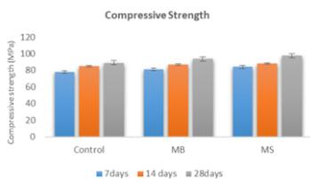
Figure 3. Compressive strength of SCHPC.
