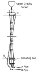
**Figure 6.** Schematic diagram of monitoring tendon duct connections during wax injection.
