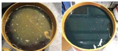
**Figure 2.** States of wax at 94°C (left) and 110°C (right).
