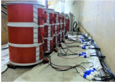
**Figure 1.** Wax melting equipment with band-shaped heaters.
