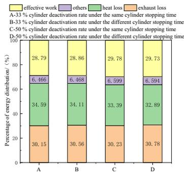
**Figure 17.** The proportion of various energy of the engine with the same cylinder deactivation rate and different cylinder deactivation strategies.
