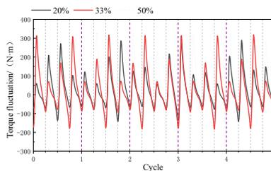
**Figure 10.** Torque fluctuation at different cylinder stopping rates.
