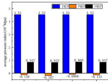
**Figure 18.** The average pressure index of the engine with the same cylinder deactivation rate and different cylinder deactivation strategies.
