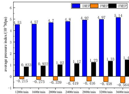
Figure 16. The average pressure index of the engine at different speeds with the same cylinder deactivation rate.
