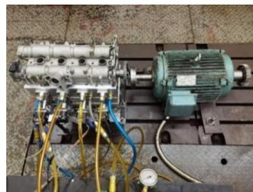
**Figure 2.** Flexible variable valve motion characteristics test platform.
