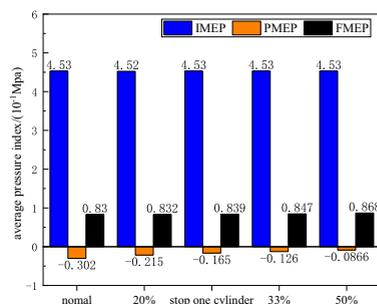
Figure 14. The average pressure index of the engine under different cycle stop rates.
