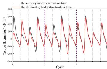
**Figure 11.** Torque fluctuation of different cylinder deactivation strategies under the 33 % cylinder deactivation rate.
