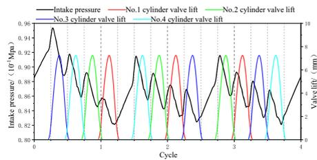
**Figure 4.** 25 % cylinder deactivation rate intake pressure.
