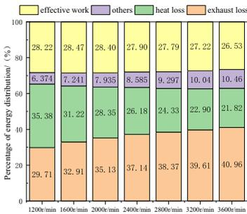
Figure 15. The proportion of engine energy with the same cylinder stop rate and different speed.
