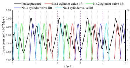
**Figure 3.** 20 % cylinder deactivation rate intake pressure.
