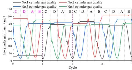
**Figure 7.** In-cylinder gas quality in 25 % cylinder deactivation rate.
