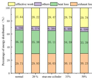
Figure 13. The proportion of engine energy with different cylinder deactivation rates.
