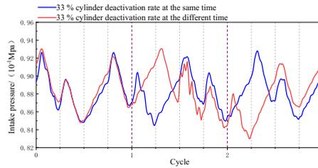
**Figure 5.** Comparison of intake pressure of different strategies with the same cylinder deactivation rate.
