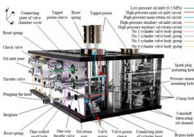
**Figure 1.** Independent research and development of hydraulic variable valve mechanism of four-cylinder engine.
