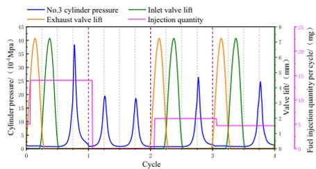
**Figure 9.** Cylinder pressure of No.3 cylinder under 25 % cylinder stopping strategy.
