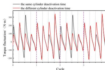
**Figure 12.** Torque fluctuation of different cylinder deactivation strategies under the 50 % cylinder deactivation rate.
