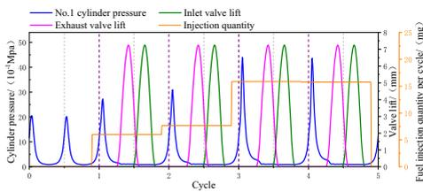
**Figure 8.** Cylinder pressure of No.1 cylinder under 20 % cylinder stopping strategy.
