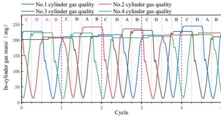
**Figure 6.** In-cylinder gas quality in 20 % cylinder deactivation rate.
