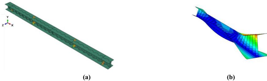
**Figure 3.** SHEA-200 model: (a) part assembly (b) global buckling mode
