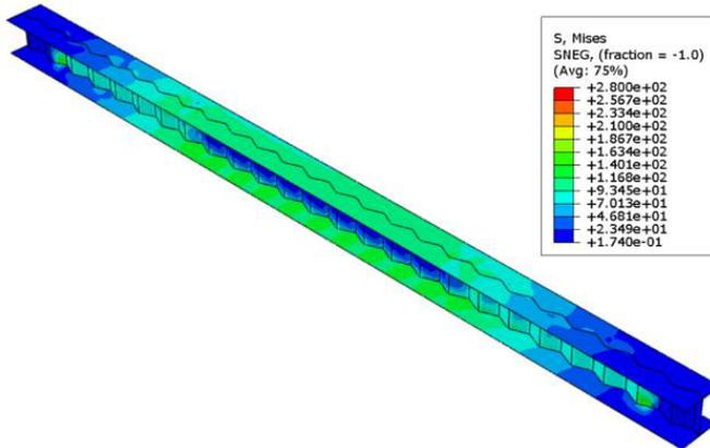
Figure 5. Stress distribution of the resulted optimized beam
