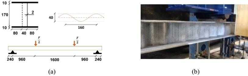
**Figure 2.** Considered SHEA-200 beam: (a) geometry of the beam (b) test layout
