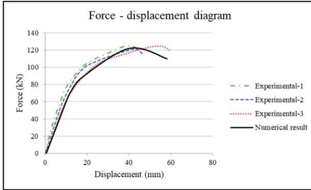
Figure 4. Force-displacement curves of SHEA-200
