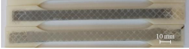
Figure 1. Injection moulded dumbbell specimens from the rear.
