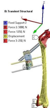
Figure 3. Types of forces exerted on pertrochanteric fixators and femur
