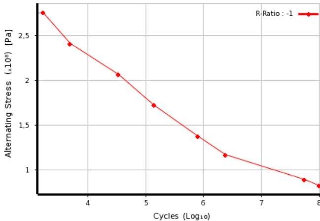
**Figure 4.** S-N curves of schanz screws having aluminum alloy [14]
