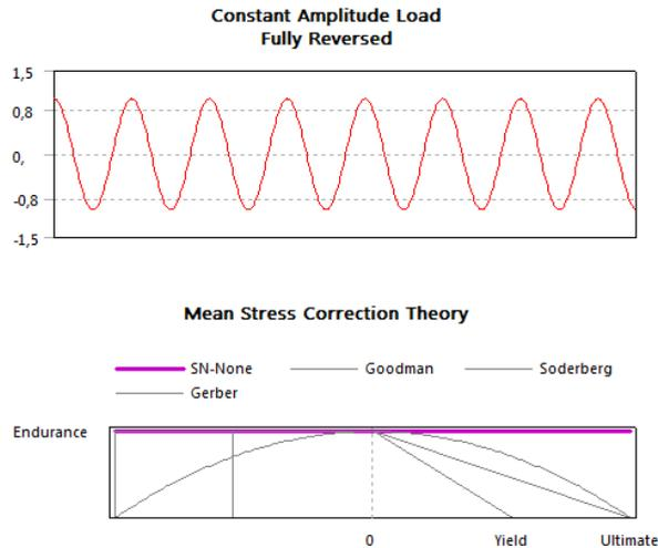
Figure 5. Fully reversed for loading type and mean stress theory
