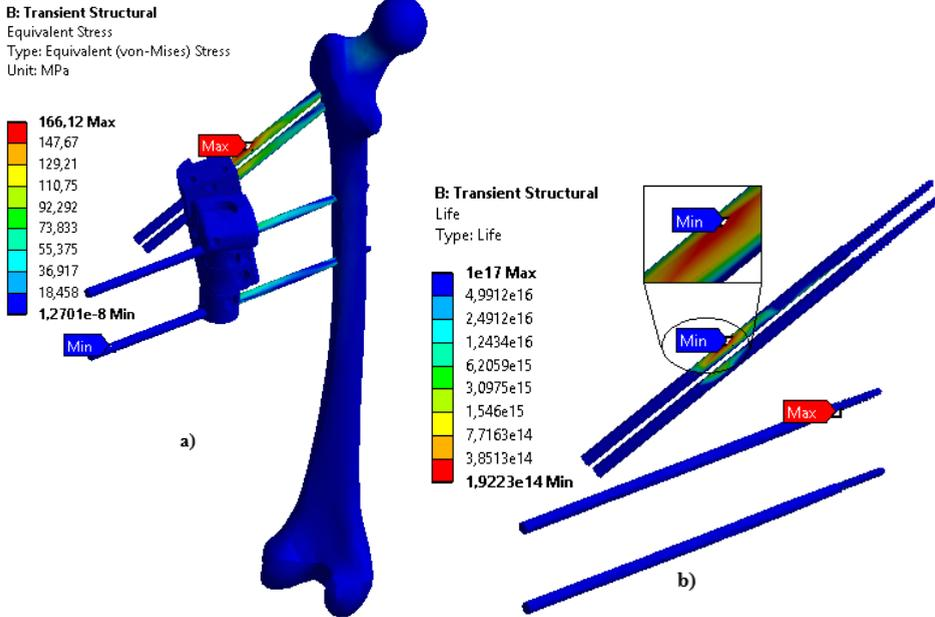
**Figure 6.** The fatigue analyse results. (a) the maximum equivalent stresses of schanz screws, (b) the life of schanz screws
