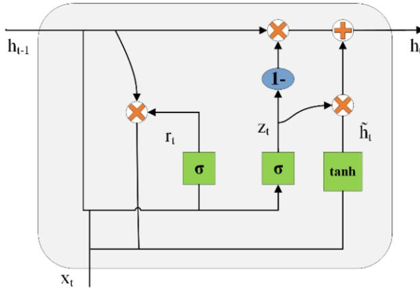
Figure 5. The internal structure of GRU cell.
