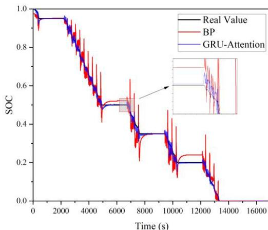
Figure 6. The actual SOC values and predicted SOC values by the two models. (DST)
