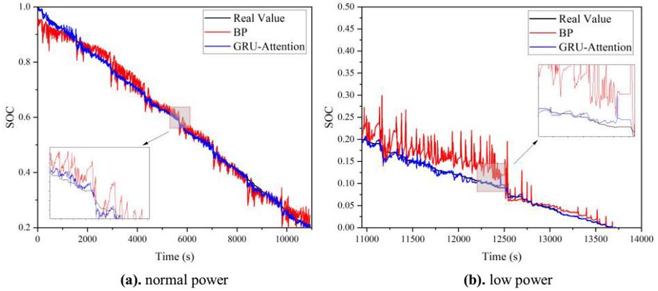
**Figure 9.** The SOC value curves under normal and low power conditions in the UDDS dataset.
