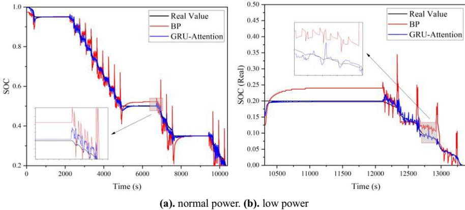
Figure 8. The SOC value curves under normal and low power conditions in the DST dataset.
