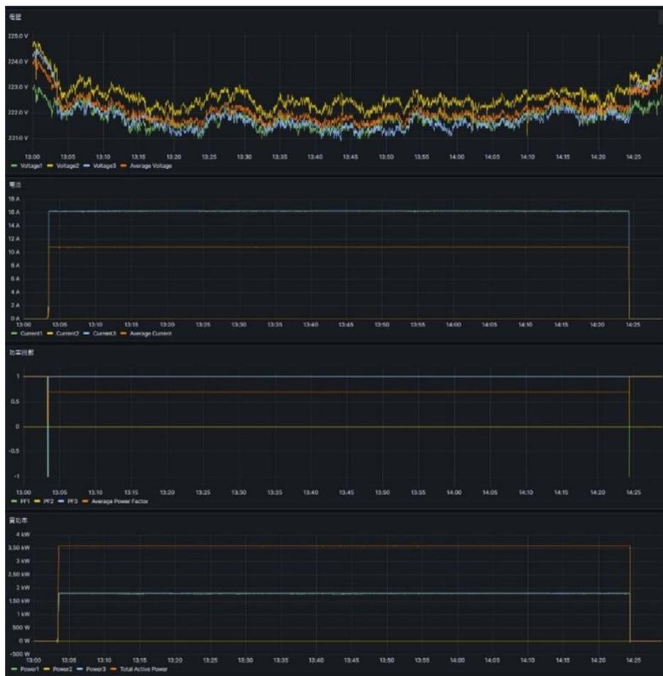
Figure 4. Test result , single-phase delta-connect line-to-line voltage is 220. (16A)
