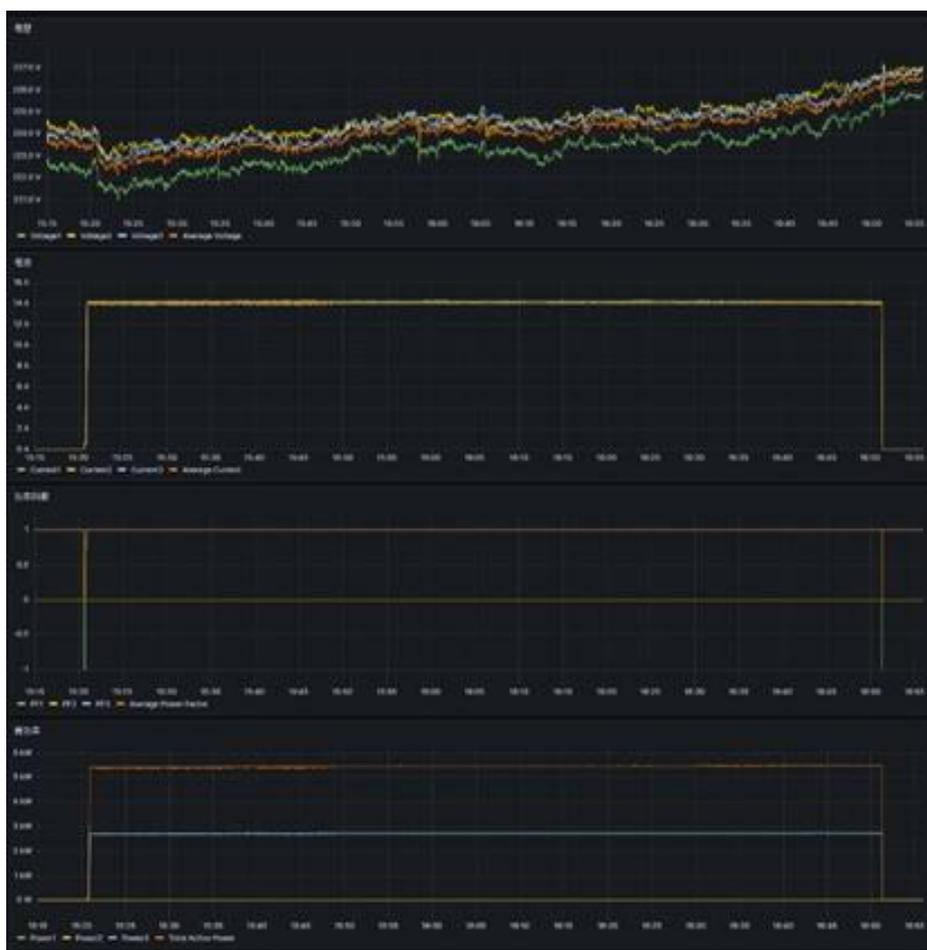
Figure 6. Test result, three-phase delta-connect line-to-line voltage is 220. (14A)
