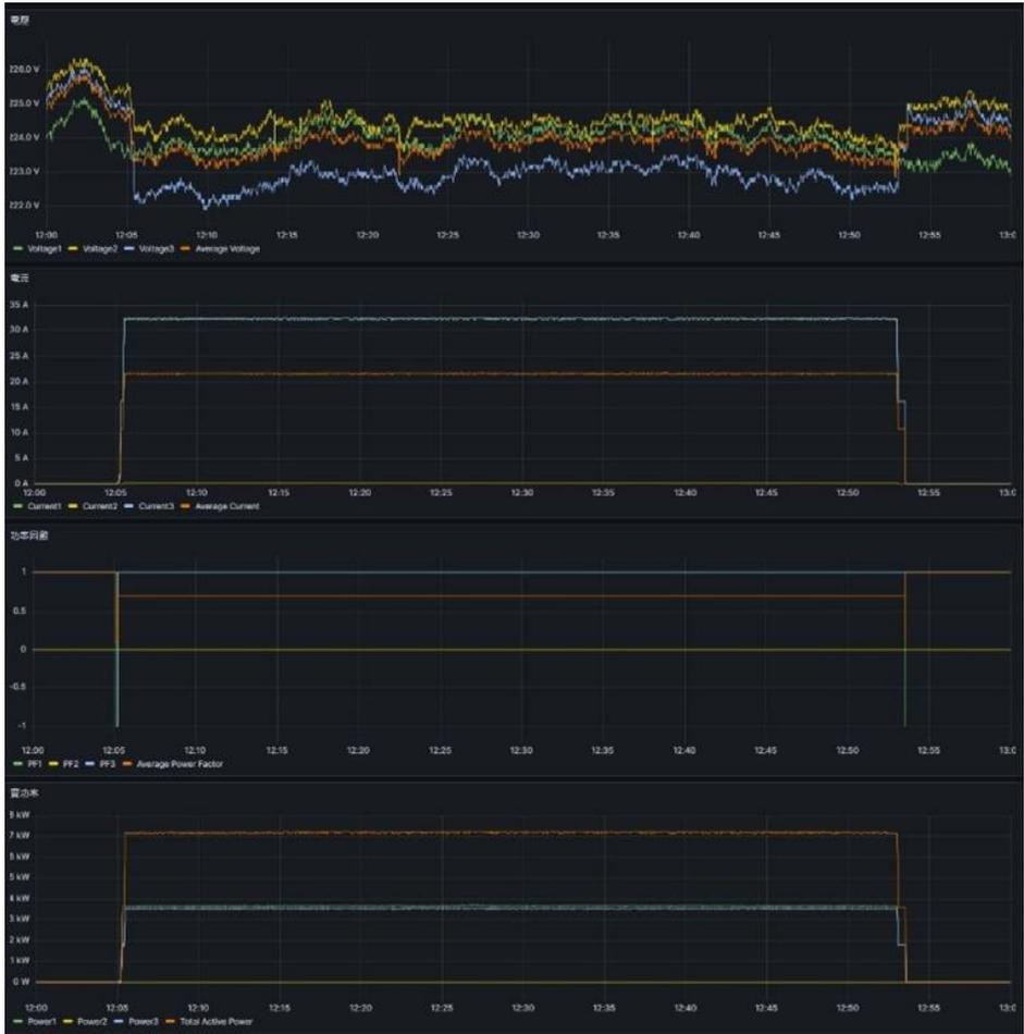
Figure 3. Test 1, single-phase delta-connect line-to-line voltage is 220. (32A)
