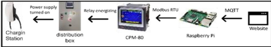
Figure 2. Hardware structure.
