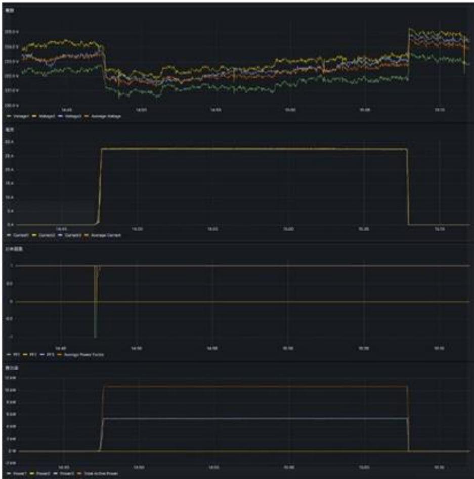
Figure 5. Test result , three-phase delta-connect line-to-line voltage is 220. (28A)
